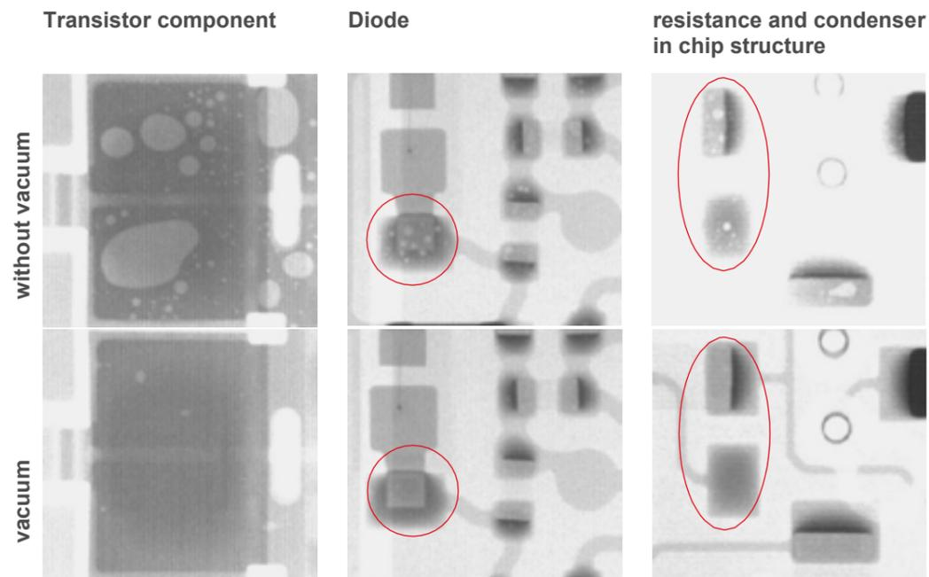
The clearly visible reduction of pore percentage was achieved in the above shown examples via the use of a reflow vacuum soldering system type SMT VAC S.
