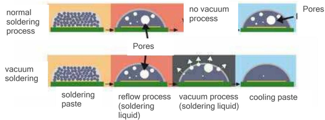
Schematic comparison of conventional (image above “normal soldering process”) and vacuum reflow processes (image above “vacuum soldering”). During vacuum reflow processes the vacuum process is programmed as the next step after the actual melting process, which extracts the pores from the liquid solder. This is followed by cooling of the component.
