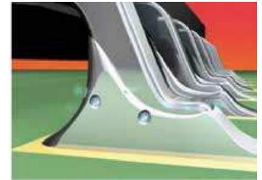
pores are extracted from the solder point in the vacuum mode
