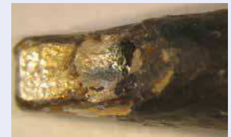
Formation of holes in the soldering tip
