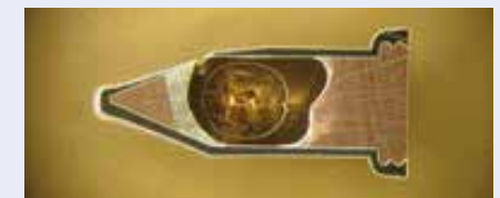
Micro-section of soldering tip with hole formation
