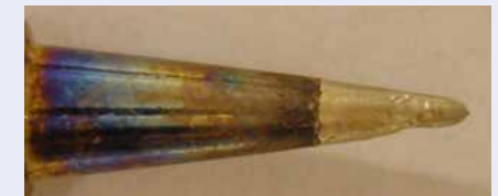
Soldering tip after 10,000 solder joints with lead-free SA
