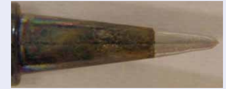
Soldering tip after 20,000 solder joints with Sn60
