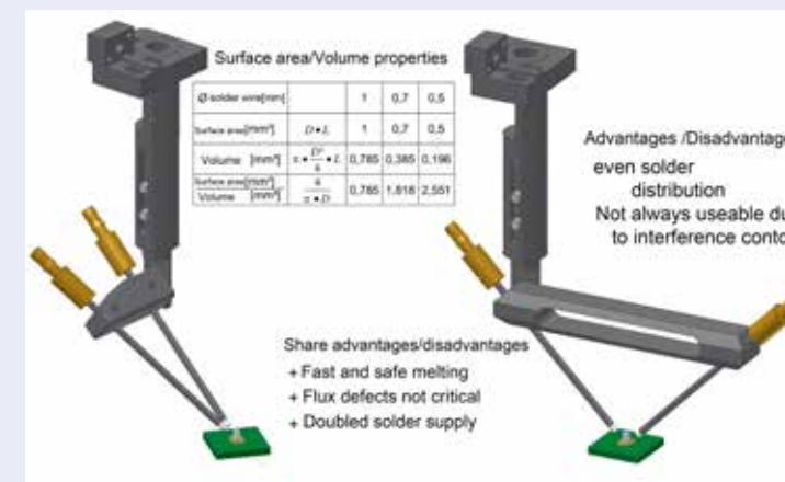
Picture 6: In place of a soldering wire usually with a 0.7 mm diameter, 2 soldering wires with 0.5 mm diameter are introduced parallel to one another
