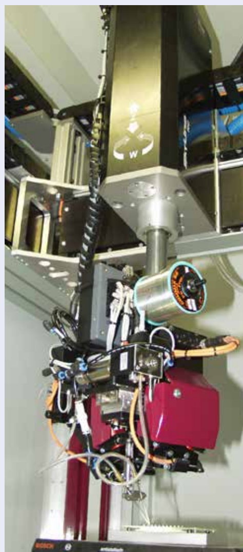
Picture 7: The laser soldering tool is positioned by a four-axle NC handling device with servo drive to the desired soldering joint.
