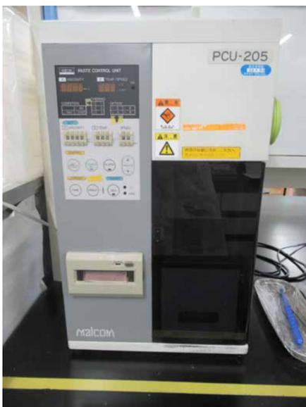
Viskosimeter / Viscometer
