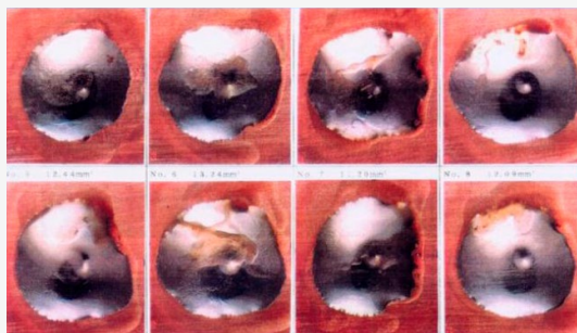
Figure 2: On the left side: Soldering points of conventional solder wire with flux core containing air pockets. Right side: Solder points of Almit solder wire with 100% continuous flux core without air pockets.
